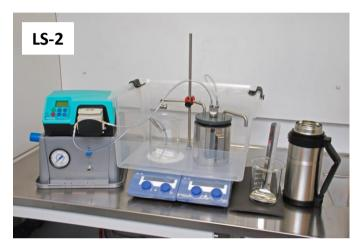
LS-2 and LS-6 consists of a slip container with a stirrer, a pump for the slip, a spray nozzle, a regulator for compressed air and an insulated chamber for spraying and granule collection.
